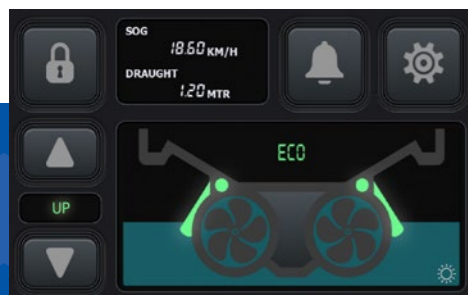
FLEX Tunnel touchscreen control panel
